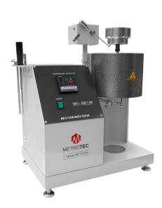
Advanced solution for determining the Melt Flow Index (MFR & MVR) of thermoplastic materials by the volumetric and gravimetric methods. It has a PID temperature controller, automatic cutting samples and software.
