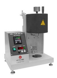
Entry level model for determining the Melt Flow Index (MFR) of thermoplastic materials by the gravimetric method. It has a PID temperature controller and automatic cutting samples.
