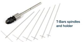
The HELIPRO device makes it possible to measure viscosity of gels, pastes, creams and more generally products that do not flowing.
