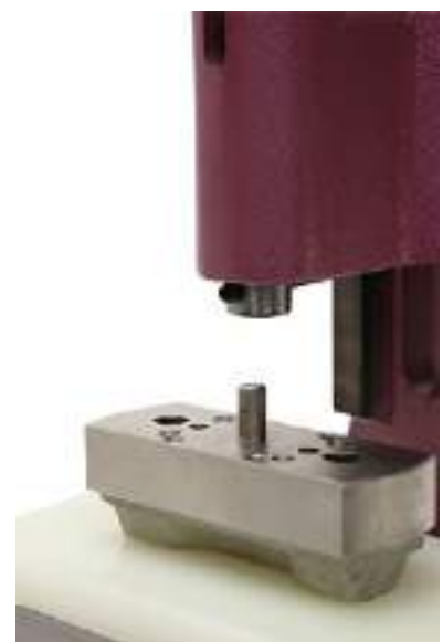
Replaceable cutter and Nylon plate
