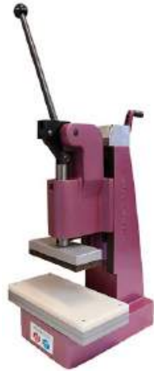
Model PCM-26 Cutting force: 26kN
