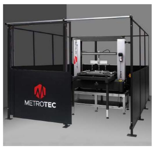
APPLICATION: Adhesion tests of components in vitroceramic cooktops.
