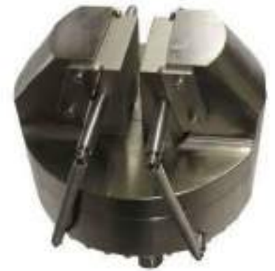
MNC/100-D260-S46 Extra wide jaw opening 46 mm
