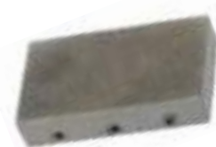
BD Diamond jaws - Clamping area covered with synthetic diamond D91 (170/200 mesh) - Nickel plated
