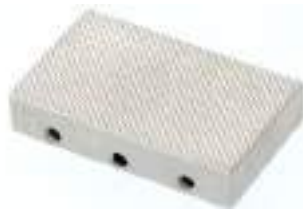
BP serrated (pyramids) - Pyramids 1.2x45 ° - Hardened steel 58 HRC - Nickel plated
