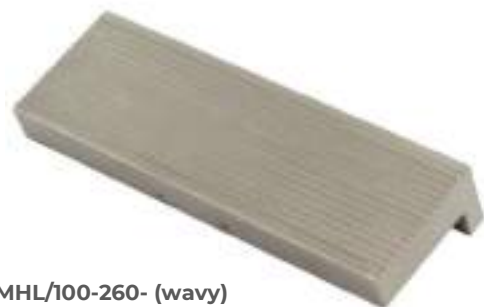
BD Diamond jaws - Clamping area covered with synthetic diamond D91 (170/200 mesh) - Nickel plated
