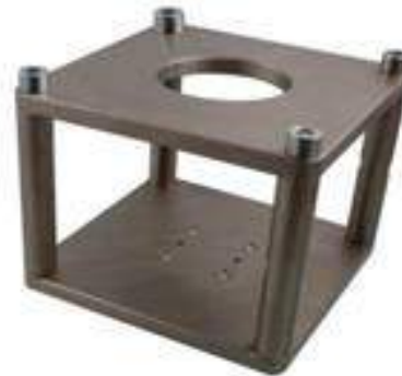
Special fixture to test withdrawal resistance of nails from wood panels (ASTM-D1037-Fig. 13 (§§13-15))
