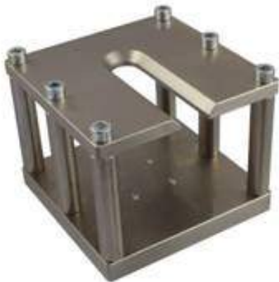
Special fixture to test withdrawal resistance of #12 screws from wood panels Maximum load 25 kN (ASTM-D1037-Fig.13 (§16))
