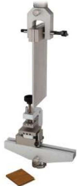
Fixture to test the tooth strength of wood laminate click systems
