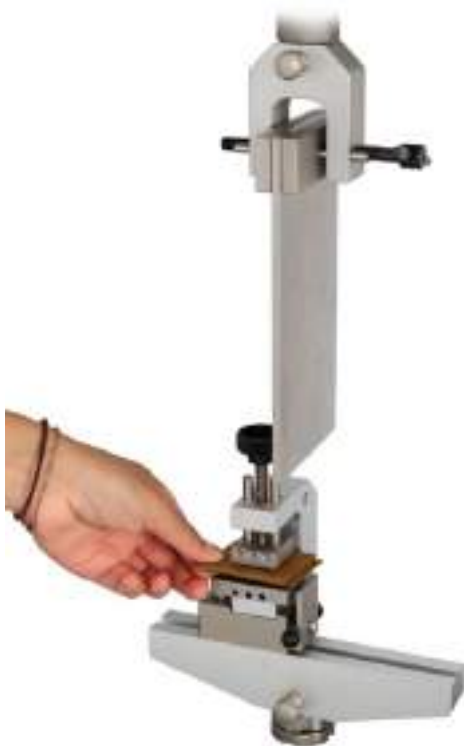
Fixture to test the tooth strength of wood laminate click systems
