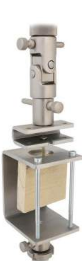
Fixture for testing parallel traction to the fiber of wood samples. (ASTM-D143-Fig.29)
