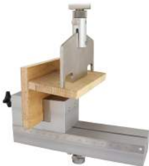
Special bend test fixture to test furniture connectors (DIN 68501)
