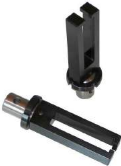
Fixture for testing parallel traction to the fiber of wood samples. (ASTM-D143-Fig.29)
