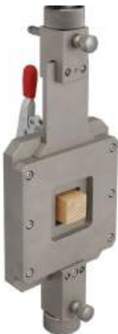
Shear Test Fixture Shear strength of adhesive bonds between rigid substrates by the Block-Shear method (ASTM D4501)
