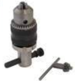
Special fixture to test withdrawal resistance of nails from wood panels (ASTM-D1037-Fig. 13 (§§13-15))
