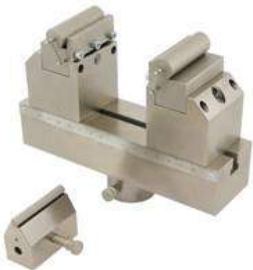
Model PFL.m / St-360 bending fixture with 360 mm bar length according to ASTM E399 to test the linear-elastic plane strain fracture toughness K IC of metallic materials
