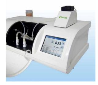
P8000-DT features temperatureа controlled micro-cuvette that can be used in flow-through operation.
