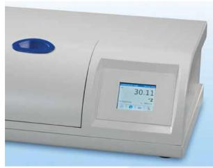
The P3000 economical polarimeter is a simplified version of the P8000 and uses the same patented fast measurement technique. It measures samples in just 1 second, regardless of the rotation angle, saving much time over measurement with conventional polarimeters.
