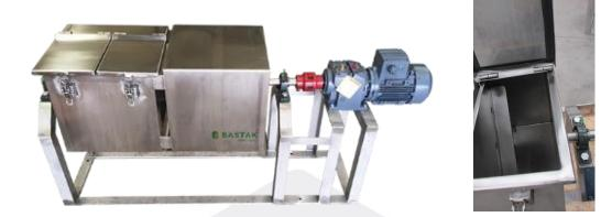
BASTAK introduces to the feed industry its new Four-Compartment Pellet Durability Tester. It is ideal for the feed mill and manufacturer to determine the amount of fines that will exist in pellets at feeding time.
