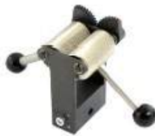
Self-clamping Grips (Elastomers - Rubber...)
